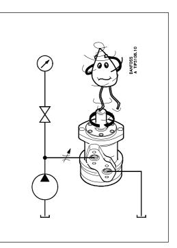
If no flow meter is available, a Danfoss hydraulic motor can be fitted instead. The displacement of the motor per revolution with unloaded shaft is very precise and to find flow all that is necessary is to count the number of revolutions per minute and multiply the figure by the displacement, as shown in the following examples:
